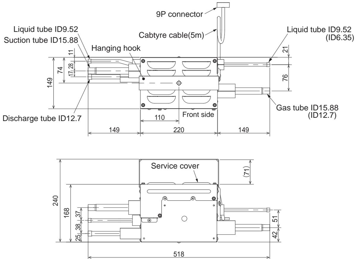
**Note:** This figure shows the unit with suspension fittings attached.
