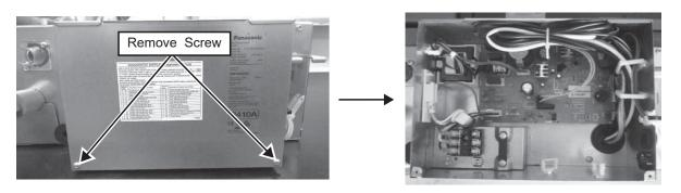
2 Detach all connectors as labeled from the electronic controller. Then pull out main controller gently.
