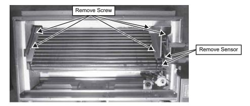
3 Unscrew 4 screws, 1 nut and 1 Spring Clip on the Drain Motor Bracket and remove Drain Motor from unit.
