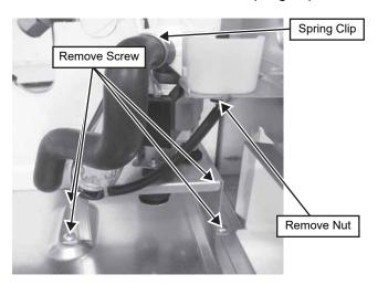
4 Unscrew 3 screws on the Drain Motor and detach the Drain Motor from Drain Motor Bracket.
