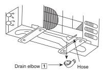
Install the hose at an angle so that the water smoothly flows out.
