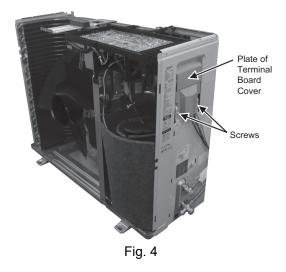
Remove the Control Board. 6
