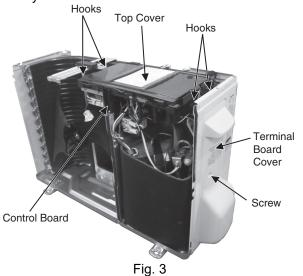
5 Remove the Control Board as follows:
