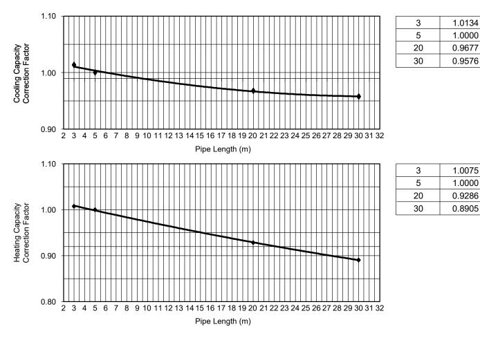
Note: The graphs show the factor after added right amount of additional refrigerant. Maximum piping length for Z25/35UBEA is 20 meters. Maximum piping length for Z50UBEA is 30 meters.
