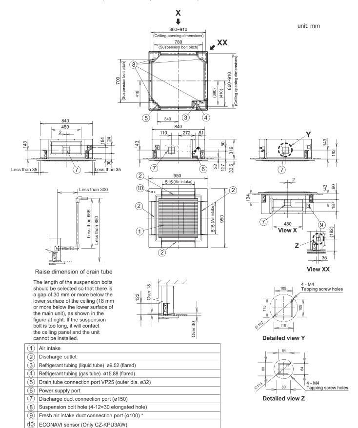
Necessary to attach duct connecting flange(field supplied).
