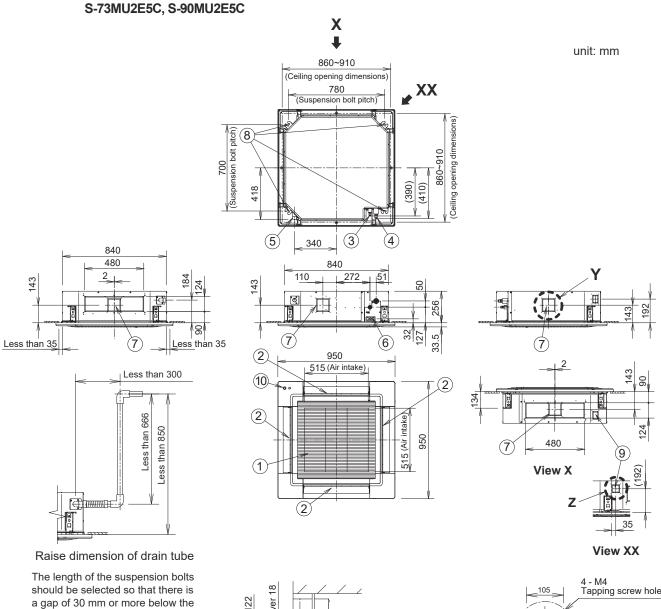
The length of the suspension bolts should be selected so that there is a gap of 30 mm or more below the lower surface of the ceiling (18 mm or more below the lower surface of the main unit), as shown in the figure at right. If the suspension bolt is too long, it will contact the ceiling panel and the unit cannot be installed.
